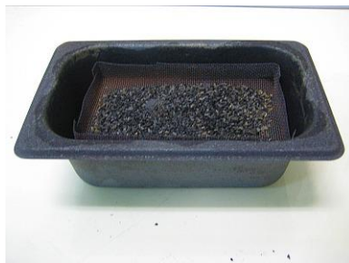
Set the reduction net Cover it, on the firing net
