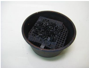
Carbon on the net for reducing material
