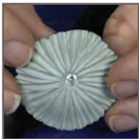
7. Bury the piece in activated carbon inside of a stainless steel firing box, or to avoid the kiln mess, use a box made from No-Flake Firing Foil. There should be at least 1/2" of carbon over the top and below the item. Program the kiln to fire at full ramp to 1425F and hold for 1 hour. When the program is complete, vent the door by opening it about an inch. When the red glow has gone from the box, remove it using tongs and place on a trivet to cool.
