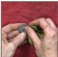
10. Use a 3M Polishing Paper in 400 grit on the front of the necklace to give a softer matte finish. The back can be polished with a 3M Bristle Disc starting with 220 grit and progressing to the finer grits to desired polish. Buff the back with a polishing cloth as a final step.
