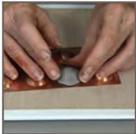
3. Place the molded clay on a drying form. Gently form the clay over the mold, pressing down the edges to conform to the mold. A Copper Drying Form is used here.
