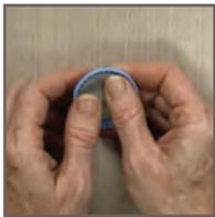
1. Make a patty from fresh clay and place into the mold. Using your thumbs with a rolling motion, press the clay firmly into the mold and outward to distribute it evenly in the mold.
