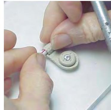
9. Using a small divit tool (ball burnisher), impress a divit at the north, south, east and west directions on the setting.
