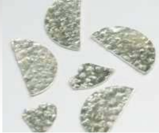
2. Pickle until the oxidation is gone.
