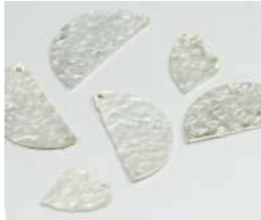
4. Pickle until the oxidation is gone.
